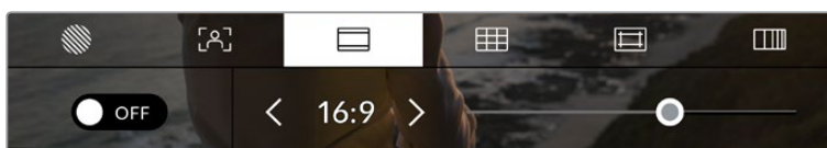
Tap the 'frame guides' icon while accessing 'LCD monitor options' to access your Blackmagic Pocket Cinema Camera 4K's frame guide settings
