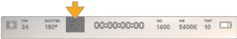
Your Blackmagic Pocket Cinema Camera 4K's iris indicator. Tap this to access iris settings
